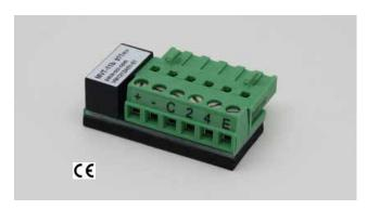
Four millivolt plug-in modules are available, each with a different millivolt range. Three of the modules (Mvt-11b, Mvt-22b, Mvt-50u) also accept a Thermocouple (Type J, K, N, R, S, T, B, C or E). A builtin, precision thermistor provides ambient temperature readings and for thermocouples, cold junction compensation.
