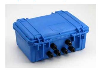
Rugged molded case withstands all weather conditions. Features a hinged cover, continuous neoprene o-ring seal, quick release latches, and fold-up carrying handle. Six feed-through cable glands accept cable diameters up to 0.25" (6.3 mm). Can be padlocked for security.
