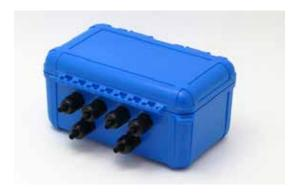
Rugged molded case withstands all weather conditions. Features a hinged cover, continuous neoprene o-ring seal and two quick release latches. Six cable fittings installed on side of case. Fittings accept cable diameters up to 0.25" (6.3 mm).
