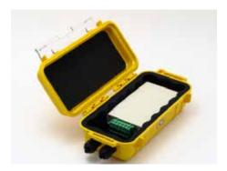
Rugged molded case withstands all weather conditions. Features a hinged cover, quick release latch, continous rubber seal and two cable fittings. Fittings accept cable diameters up to 0.25" (6.3 mm). Available in Black only. Yellow case pictured above is no longer available.
